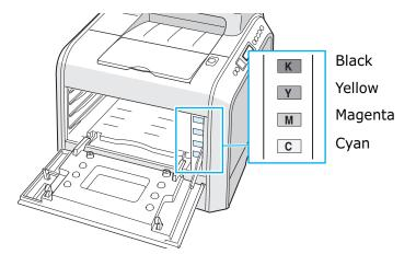
14 Holding each toner cartridge, insert them into their corresponding positions in order of Cyan, Magenta, Yellow and then Black. Using both hands, grip the cartridge to insert into the slot. Then hold the handle to slide the cartridge in.
